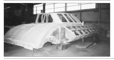
However the result, 10ft x 12ft, is smaller than any wing deck cabin you have ever seen on a cat this size, especially considering it will do duty as the saloon-galley-helm station. The hulls are as narrow as possible (3.3ft at WL). When it was time to do the fibreglass taping inside the focsle, the entry was so tight one's head would get stuck. As a result, we have the accommodation space of a 40-foot cat on 63-foot hulls and our interior definitely looks like an
